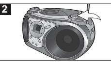
Tune a desired station by turning the TUNING control.
